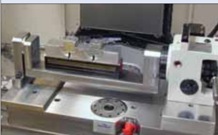
Solution: Rotary table fixtured with a zero-point docking system for repeatability.
