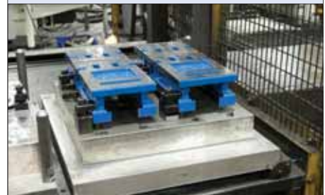
Solution: Grinding fixture increases holding power and improves accuracy.
