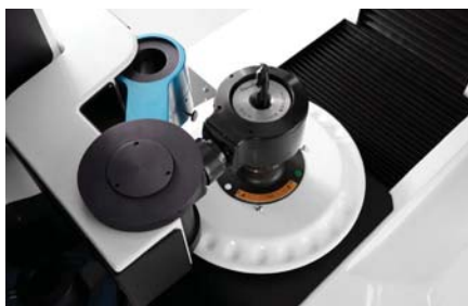
Standard Coil to Shrink HSS Tools from 3-32mm in Diameter
