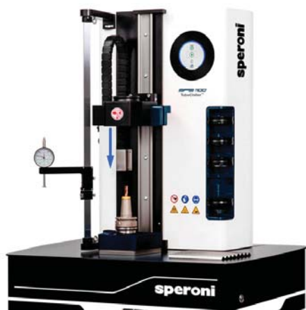
The High Frequency Coil Heats Up the Tool Holder
