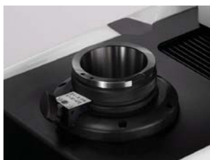
High Precision ISO 50 Spindle
