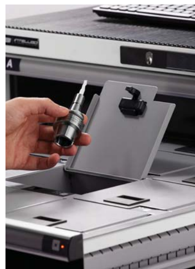
LED Lights Indicate Storage Location
