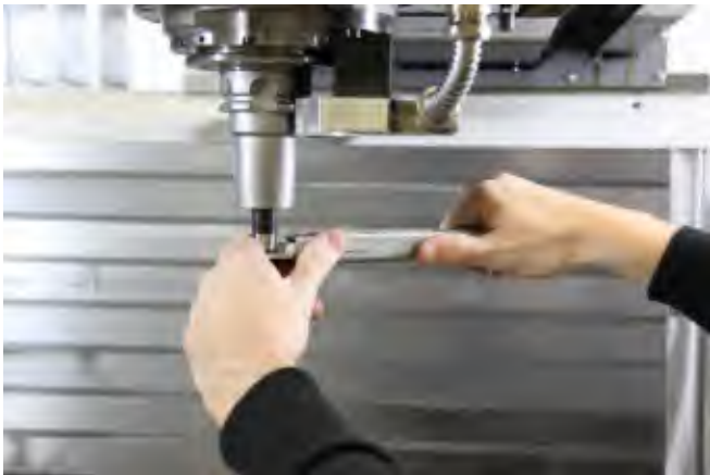
Additionally placing a hand on the exchangeable milling head is important for sensitive alignment. This helps to ensure the torque can be better maintained.
