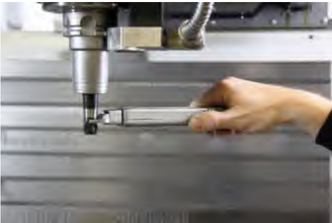
The torque key must be horizontally aligned with the key face; take care not to tilt the key face.
