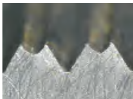
Underformed – core hole too large
