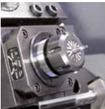
The locking mechanism holds the tool in the base
