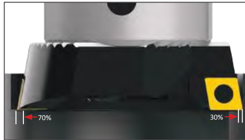
Material removal up to 7.00 mm - 10.00 mm (0.276" - 0.394") on diameter: 70% roughing 30% finishing
