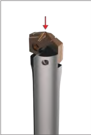
Step 2: Slide the insert into the precision ground locating pocket on the holder. The insert should not be turned, rotated, or twisted for locking purposes. The holder pocket and locating pads on the insert assure optimum fit and repeatability.
