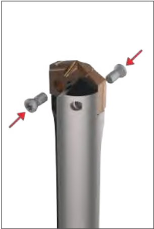
Step 3: Apply a generous amount of E-Z Break® (provided in the packaging) onto the supplied TORX® Plus screws. Tighten the TORX Plus screws to the recommended torque value specified in the catalog by series. A preset TORX driver is available to assure that the proper torque is applied.
