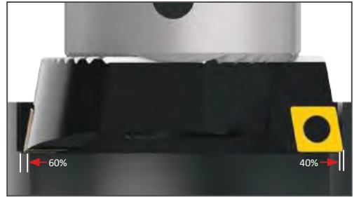
Material removal up to 4.00 mm - 7.00 mm (0.157" - 0.276") on diameter: 60% roughing 40% finishing
