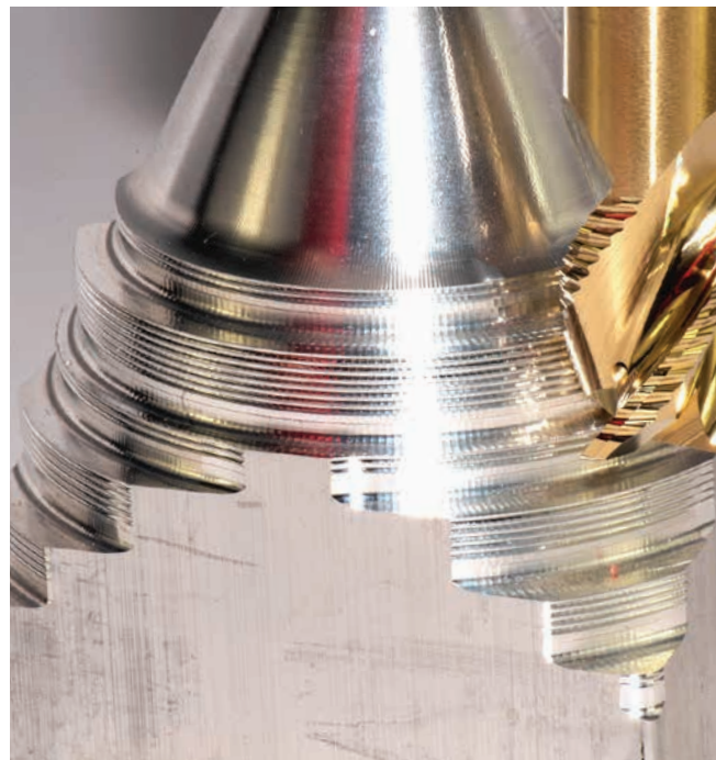
ZRN coating enhances tool life and chip evacuation.
