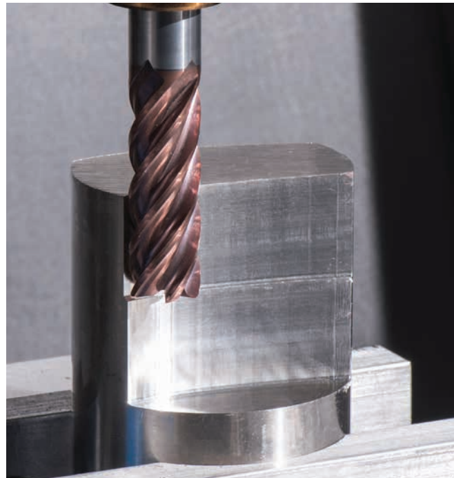
ENDURASpeed Red coated 4 or 5 flute design for High Efficiency Machining (HEM) heavy profiling.
