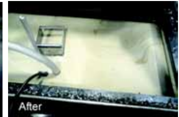
Flexor in action, with Sumpster, removing tramp oil (and a glob of biofilm), cleaning this neglected sump in under two hours.
