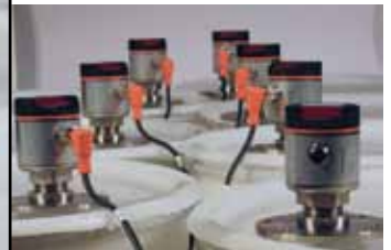
Level sensor array shown here being tested on simulated sumps before installation.
